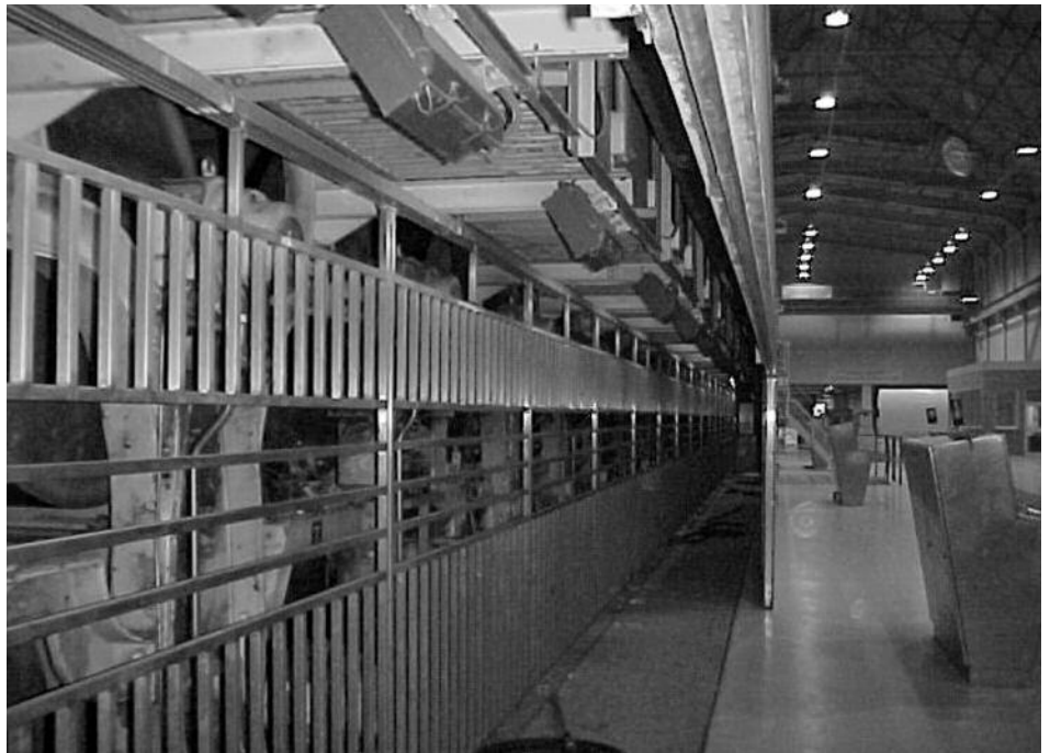
Figure 24 Guarding should be as close as practicable to the machine to prevent whole body access between the guard and machine frame
