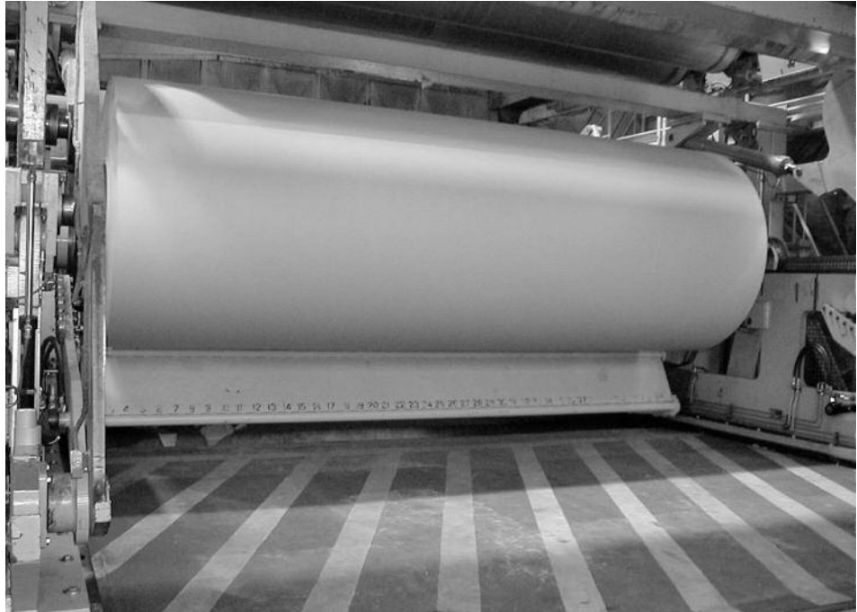
Figure 28 Drum (Pope) reel with guard at under-machine pulper
