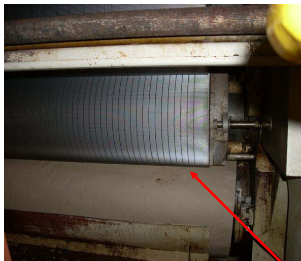
Fingers amputated between Lower Corrugator Roll and Press Roll.
